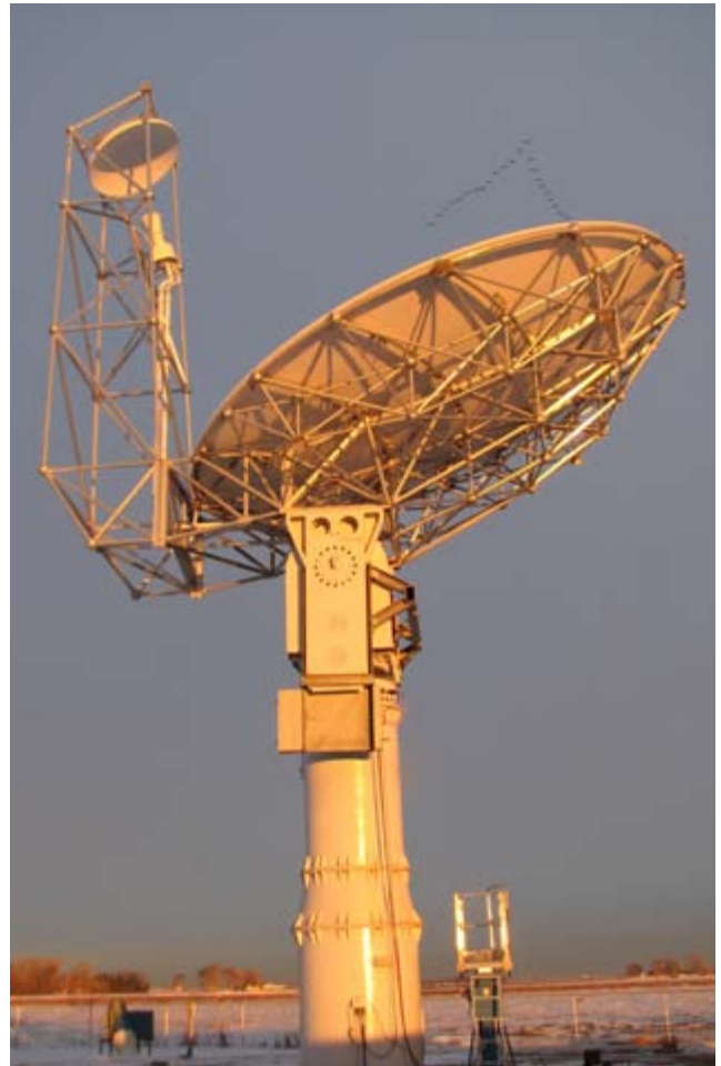
CSU-CHILL's 9-meter dual-polarized, offset-fed S-band Antenna receiver bandwidths.
