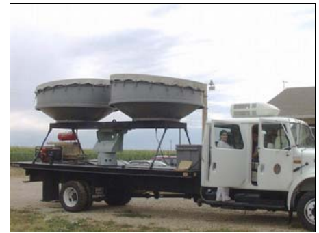
Figure 3: Vertically-pointed, bi-static, S-band FMCW radar from the University of Massachusetts (UMASS). This radar provided the backscattering characteristics of the clear air boundary layer. During the bi-static experiment involving the CSU radars, the antennas of the CHILL and Pawnee systems were positioned so that their beams intersected above the UMASS
