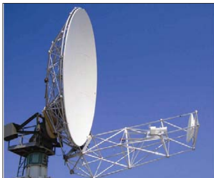
Figure 2: The offset feed antenna mounted on the positional at the Vertex/RSI test range.
