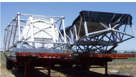
Figure 6: Feed boom and center main reflector section of the new antenna.
